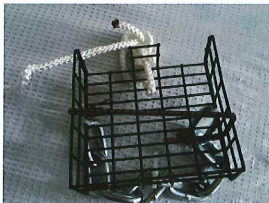
Figure 3. Bridge sampling device provided for Butler County Stream Team volunteers.
